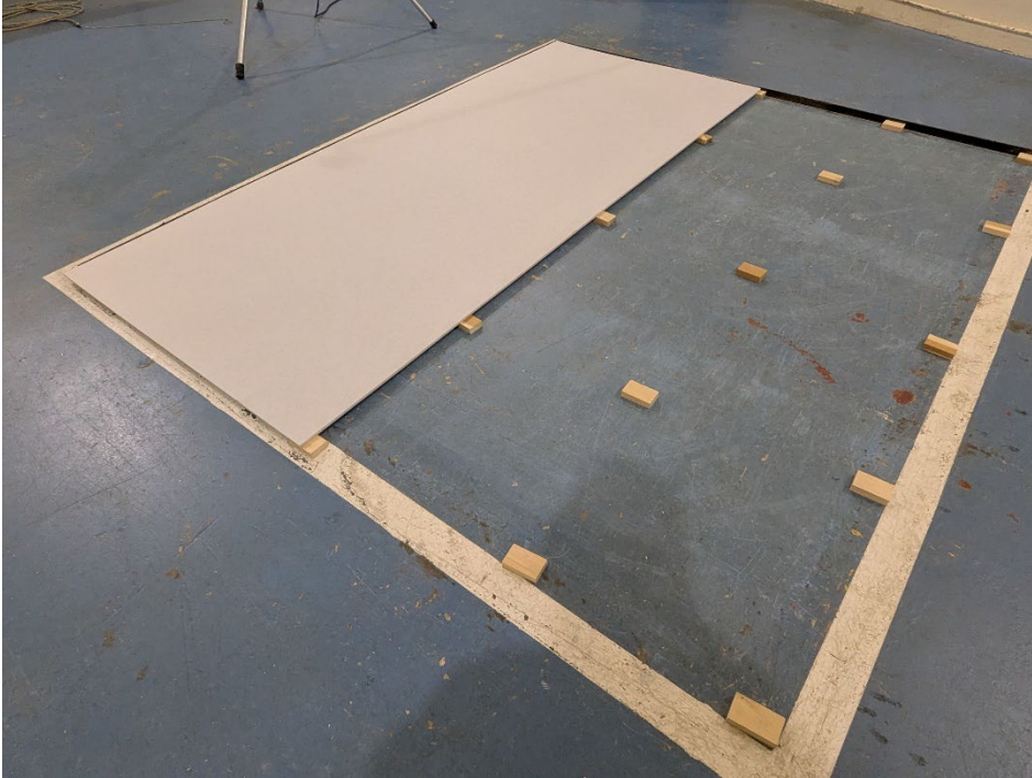
Figure 3 – Specimen partially installed over spacers
